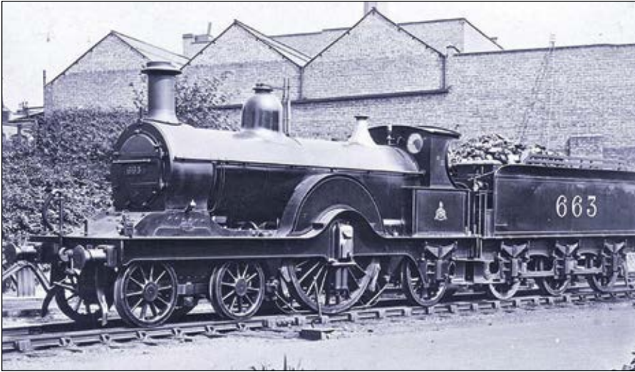
Plate 15. The elegant 4-2-2 'Spinners' of the Midland Railway were designed by Samuel Johnson. This particular example was built in Derby Works in 1893 and is marked appropriately on the wing plate beneath the smokebox saddle. The Midland Railway Arms on the cab sheet and the number '663' show that the photograph was taken after 1907, as the locomotive was originally '182'. From a pre-1914 photograph in the author's collection.
