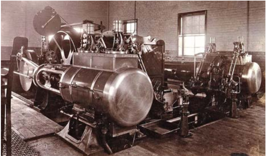
Plate 2. A twin horizontal-cylinder mill engine by Robey & Co. Ltd of Lincoln, fitted with patent drop valves and marked accordingly. These engines bear the order-book numbers '28711' and '28712' on the end of the valve chests above the cylinders; other examples of this general type, however, will bear names—commonly taken either from classical mythology or provided by the wives and daughters of mill owners and local politicians.
