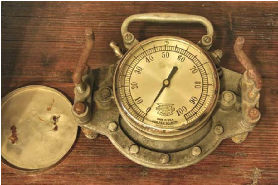
Plate 36. The dial of this pressure-test gauge by the Crosby Steam Gage & Valve Company of Boston clearly shows the shield-like trademark. Canadian Museum of Making collection.
