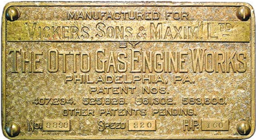
Plate 17. This historically significant plate was recovered with the wreck of Holland No. 1 , the first submarine to serve the Royal Navy. Though the power-plant has often been identified as a Wolseley petrol engine, the plate confirms that an American-made Otto gas engine was being used at the time of loss (1913). By courtesy of Ian M. Clark.
