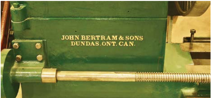
Plate 24. This manufacturer’s mark is cast into the bed of a sliding gap-bed lathe of c. 1900, from the Pictou shipyard in Nova Scotia. Museum of Making collection.
