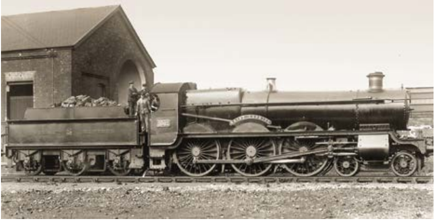
Plate 26. the Great Western Railway 4–6–0 no. 2922 Saint Gabriel , built in 1907, poses ‘on shed’. Note the cast-brass nameplate above the centre driving-wheel splashers, which can serve to identify the locomotive (one of a class of 190) if the comparatively small number plate on the cab sheet is hidden or indistinct. Author’s collection.
