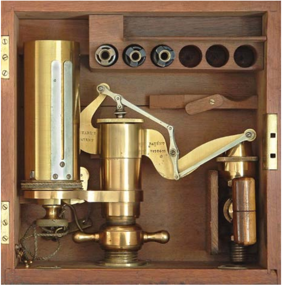
Plate 29. This Elliott-Richards engine indicator, made about 1875/6, is marked 'Richards Patent No. 10411': the 10411th instrument made under the terms of the original licence.
